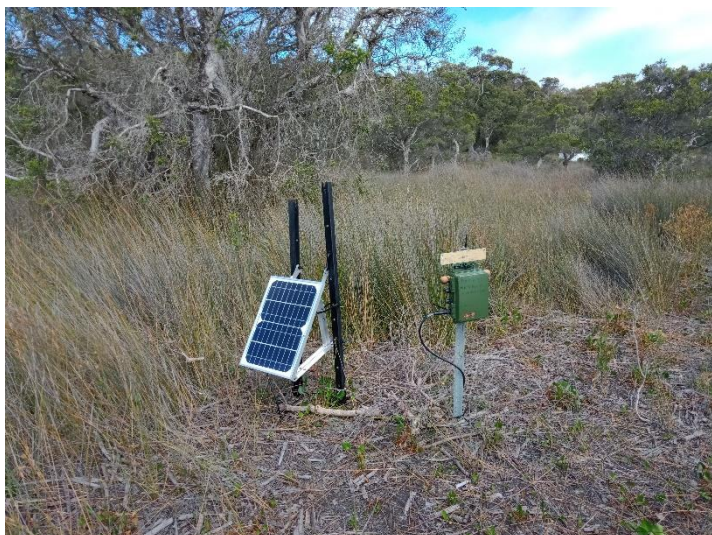
Figure 1: SM4 Song Meter and solar power source set up on the fringe of Lake Pleasant View.
